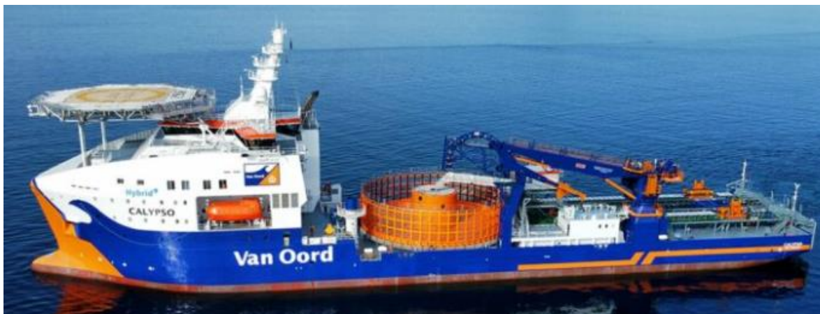
Figure 13 Cable laying vessel (source: Van Oord)
